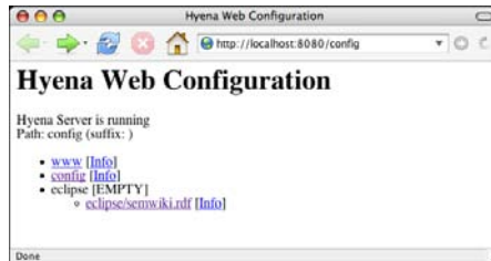
Fig. 11. HYENA’s document hierarchy: First is a container www that serves static web pages, second is the configuration container config , last is an Eclipse container with all currently open documents (currently, only “semwiki.rdf” is open). Every container is accessible via its URI, for example, you are currently seeing the answer to a GET request to the configuration container.
