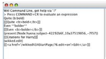
Fig. 10. An interactive session with the WITL command line: We evaluate bold markup in two variations; present a prettified version of a wiki page node; and show how editing is added to a page (it can be added to sets of pages via a skin). Note that one can make out in the produced HTML that the start page is currently selected in HYENA. Output is shown as it would be encoded in WITL.
